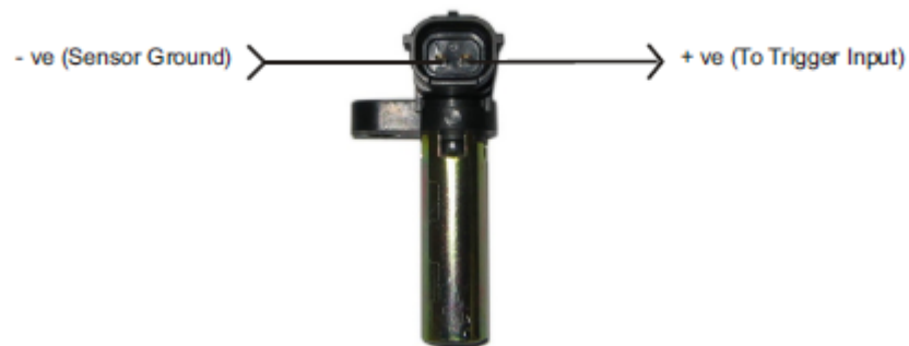
Subaru EZ30R (H6) Crank Angle Sensor Wiring
